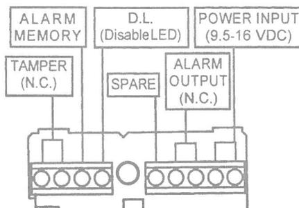
**[ Connect tamper terminals to a 24 hour supervisory loop. ]**
