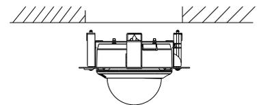
⑤ Screw up the butterfly clamp in clock-wise and clamp the bracket to the wall
