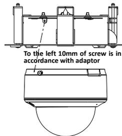
④ Insert the dome camera and bracket to the wall
