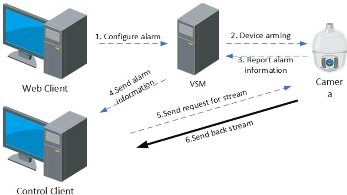
**Figure 3-12 Flow of Obtaining Alarm Related Stream Directly**
