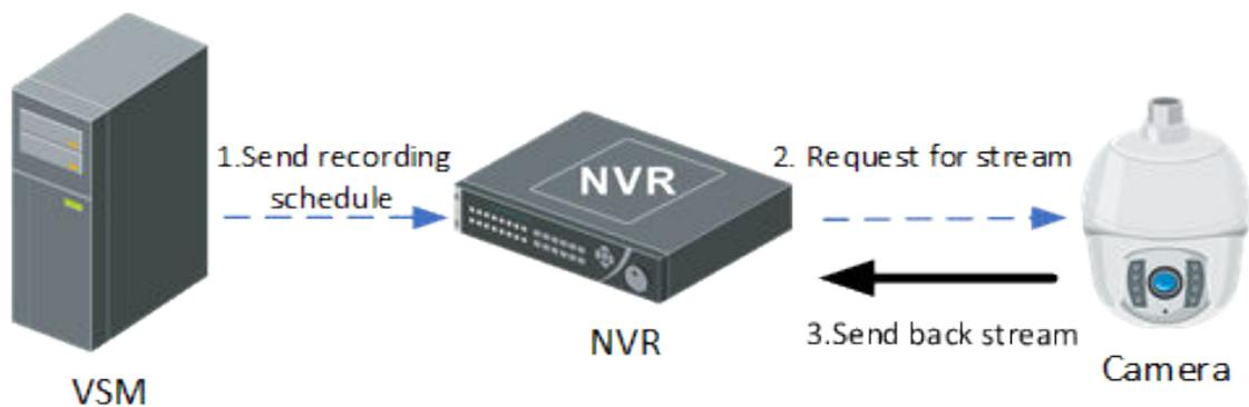
**Figure 3-6 Flow of Video Storage in NVR/DVR**
