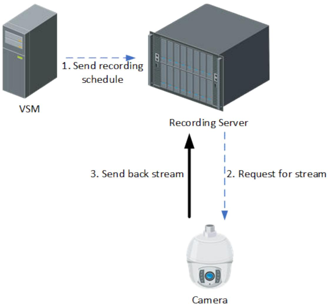
**Figure 3-7 Flow of Video Storage in Recording Server**
