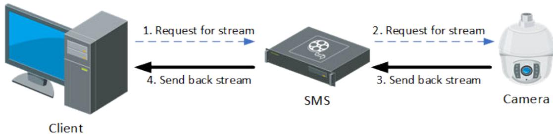
**Figure 3-3 Flow of Live View via Streaming Server**
