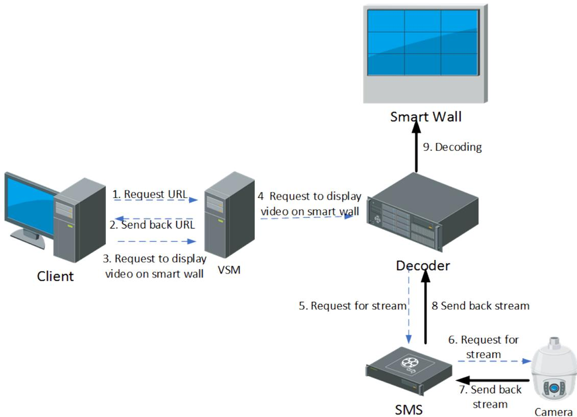
**Figure 3-15 Flow of Displaying Video on Smart Wall via Streaming Server**
