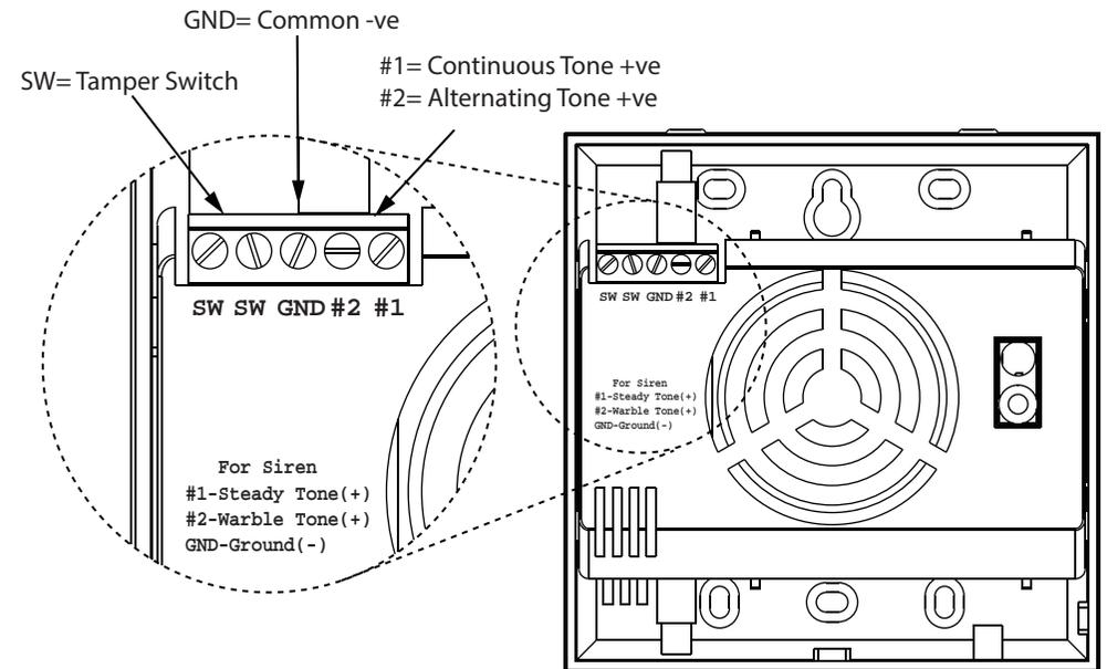
There are five terminals for the connection of wires as shown above. To activate either the alternating or continuous sound, connect a negative to the common negative terminal (GND) and connect a positive to the appropriate positive terminal (#1 or #2). To stop the sound, remove the positive or negative supply.
